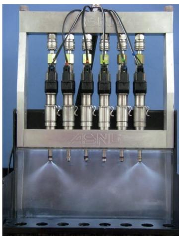
ASNU's engineers then looked at the ability of testing the injectors at systems pressure. Producing a system that could safely show the operation of the injector at high pressure was not a problem, but seeing exactly what the injector was physically doing at high pressure when compared to low pressure testing made the high pressure function more of a disadvantage than a benefit.
