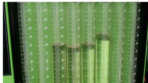
Developments in the Engine Management System now mean it can adjust the flow rate to the individual injector and compensate for any deficiency in the injectors ability to deliver the correct amount of fuel. In theory this is ideal, in practice it's not. This feature is not correcting the problem, it is compensating for it and although in the
